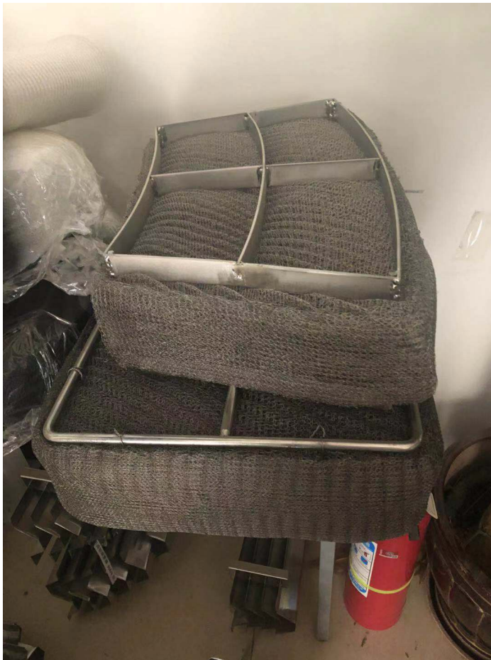
Figure 16: Mist elimination mesh pad to be installed in the China facility
